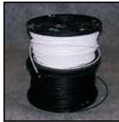
Raven Welding Rod is used for field seaming, repairs and detail work, such as installing pipe boots. Packaged in 25 lb spools, it is available in 4mm and 5mm sizes to fit most brands of extrusion guns. Raven Welding Rod is made from a thermally UV stabilized LLDPE resin and is available in both black and white to correspond with the color of geomembranes being utilized.
