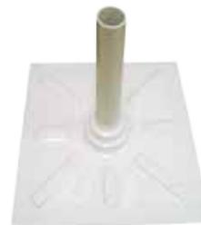
VaporBoot Plus Preformed Pipe Boots are produced from heavy 40 mil co-extruded polyethylene and barrier resins for excellent strength and durability. The preformed boots are stepped to fit 1" to 4" wide pipe penetrations. VaporBoot Plus Preformed Pipe Boots are available in quantities of 12 per box.
