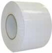
This white single-sided tape combines a heavy-duty, weather-resistant polyethylene backing with an aggressive rubber adhesive. VaporBond Tape offers excellent seaming capabilities for our materials with an "Easy Tear" feature to reduce installation time. TVB4 has a WVTR of 0.18 perms per ASTM D3833. Typical applications include vapor retarders, covers and liners. Available in 4" x 210' roll.
