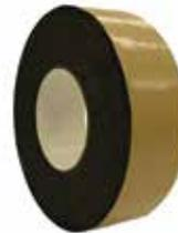
Butyl seal is a double-sided reinforced aggressive black butyl rubber tape used to join panels of polyethylene and polypropylene together by overlapping the edges and applying Butyl Seal in between. It is also used to adhere to concrete walls and footings when properly prepared. Butyl Seal is non-hardening and flexible. Available in 2" x 50' roll.
