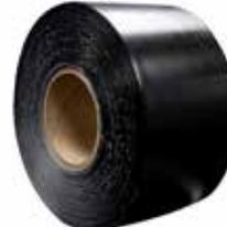
R25B Tape is a single sided aggressive synthetic elastomeric adhesive that bonds instantly to properly prepared polyethylene and polypropylene. The black polymer backing and adhesive is specially formulated to provide years of performance even in direct sunlight. A poly release liner provides for ease of installation. Available in 4" x 100' roll.
