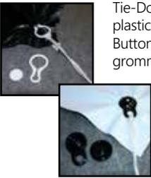
Tie-Down Buttons & Tarp Grabbers help keep plastic sheeting securely in place. Tie-Down Buttons are designed to eliminate traditional grommets in plastic sheeting up to 10 mil thick and are reusable plastic fittings that are easy to install in any position. Tarp Grabbers are up to 4 times stronger than a brass grommet and are typically used in heavier plastic sheeting from 10 mil to 30 mil thick. Great for equipment covers, large storage covers and truck tarps.
