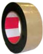
VaporBoot Tape is a single-sided elastomeric butyl tape used to complete pipe boot installations (sealing the boot to the pipe). The 100% stretchable Butyl adhesive features excellent adhesion values and 3-D stretching that can be easily molded to multiple surfaces without any creases and folds. Available in 2" x 16.4' roll.
