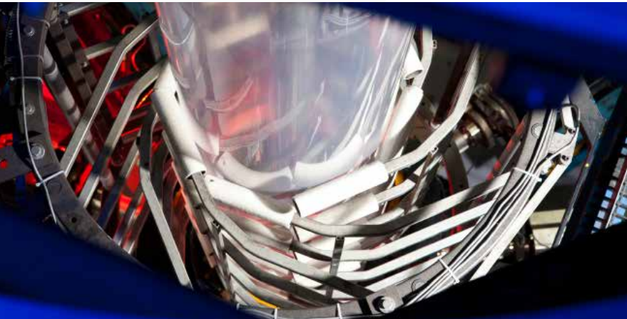
▲ View down from the upper deck of our 9-layer extrusion pilot line capable of producing a broad range of blown film/sheeting design formulations.
