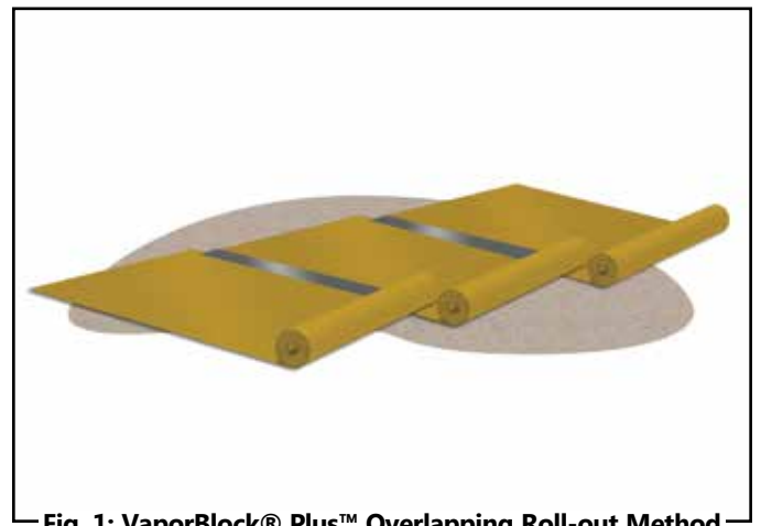
Fig. 1: VaporBlock® Plus™ Overlapping Roll-out Method
