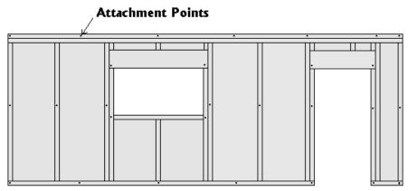
Apply a small bead of polyurethane caulk to each vertical and horizontal metal stud. Attach the **DURA** "**SKRIM** Vapor Retarder to metal studs along the top of the wall with fender washers and a self taping screw or pop rivet (see drawing for spacing) working down to the bottom of the wall.
