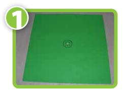
Trace or measure the pipe size onto VaporBoot G material. Cut a hole approximately 1/2" smaller than outside diameter of pipe. Make several 1/4" long cuts from inside of hole in four to eight places depending upon size of pipe. This will allow pipe to fit tightly in the hole and VaporBoot G to stretch around the pipe.
