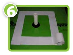
Finish VaporBoot G installation by taping exterior edge of the boot down onto VaporBlock<sub>®</sub>G<sup>™</sup> vapor retarder with Raven VaporBond seaming tape (sold separately) or an approved equal.
